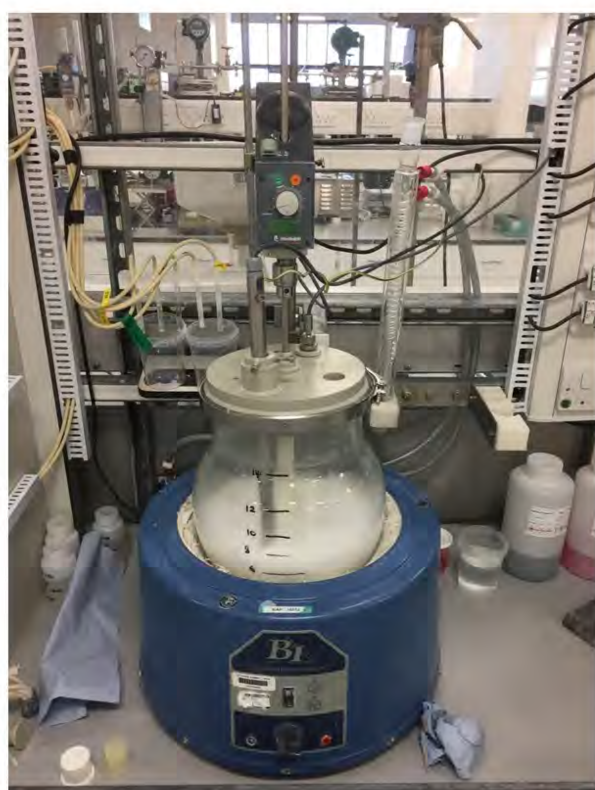
Titanium dioxide coating rig.
