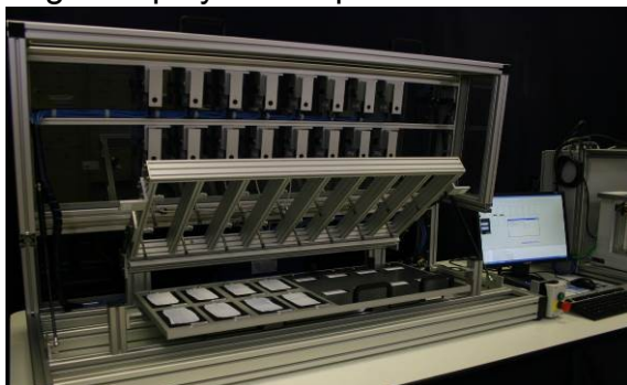
An automate scrub and burnish resistance testing system.
