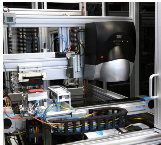
Inside a coatings analysis system: Showing a spectrophotometer, gloss meter and temperature and humidity monitoring.
