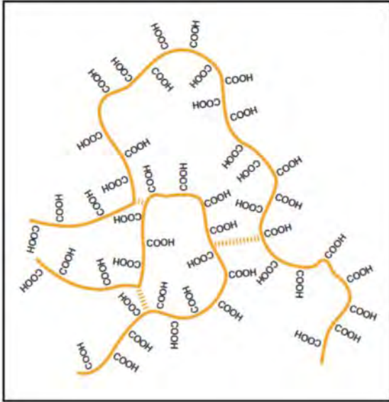
Figure 1 Schematic drawing of a molecular segment of a cross-linked polyacrylic acid polymer
